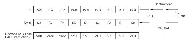
Fig. 2-1 Relationship between the PC, the Stack, and the Operand of BR and CALL Instructions
